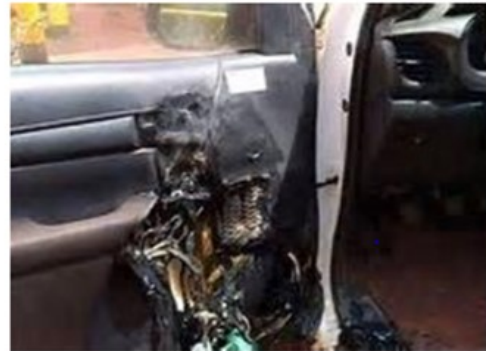
This picture shows damage to a car as result of hand sanitiser fire
